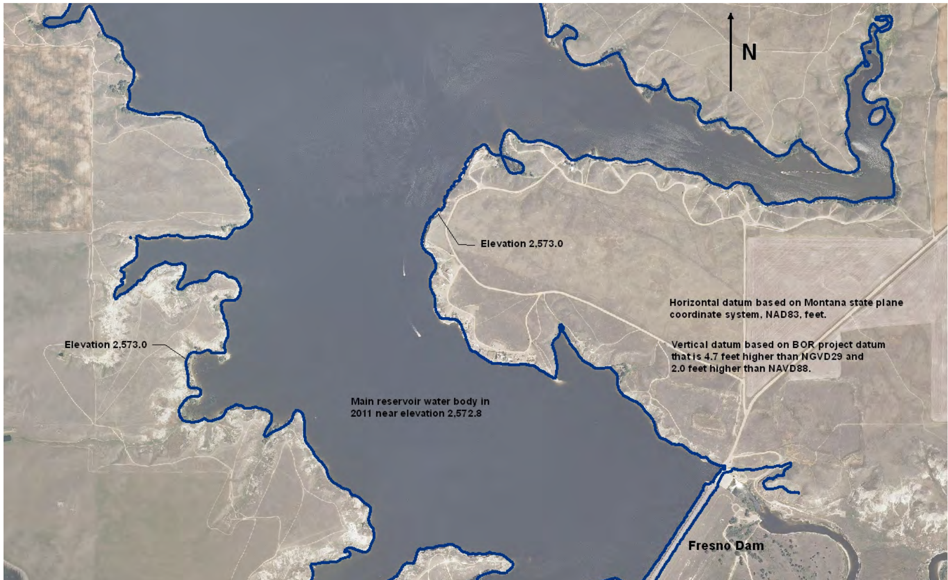
Figure 7 - Fresno Reservoir, 2011 USDA aerial photograph flown at water surface elevation 2,572.8 and the IFSAR developed contour at elevation 2,573.0 (1 of 2).
